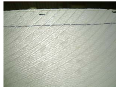
Figure 8. Replica wing made out of nylon monofilament emulating actinofibrils vacuum-bagged on polyester rip-stop cloth
